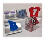
This is a new project to Year 9; a device stand that has been formed by shaping and folding a piece of sheet aluminium after firstly developing the design through modelling and prototype work.
